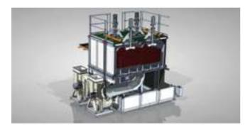
Water, water/polymer or oil tanks are designed taking advantage of computed fluid dynamics in order to optimize flow around actual load shape. Different water flow direction solution (horizontal/vertical) with Kaplan duct fans or diffuser nozzles under the load are available. Quenching can be performed: with the load still sustained by the fully integrated loading machine, with
