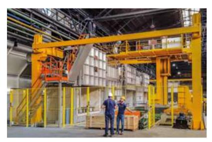
**5** batch furnaces in nitrogen atmosphere with radiant tube heating elements
