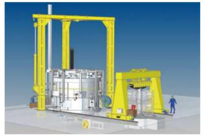
Heating is performed by high speed gas burners with heat recovery from exhaust gasses
