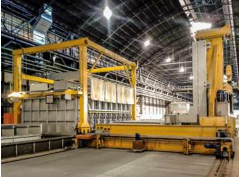
Direct immersion in quenching tank in less than 30s
