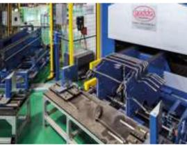
The furnace is integrated in the customer's automatic production line and fed by robotic arms
