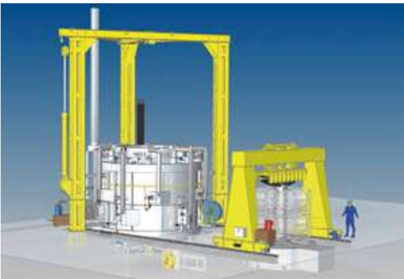
**Heating is performed by high speed gas burners with heat recovery from exhaust gasses**
