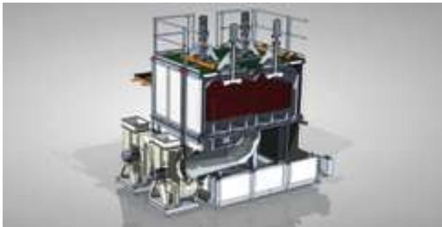
in order to optimize flow around actual load shape allowing fast and uniform controlled cooling. Cooling rate can be controlled in feedback through inverter powered recirculation fan. Isothermal annealing treatment chamber are manufactured. When forced cooling is not needed, free air normalization stations with optional smoke aspiration and thermal shields are offered.
